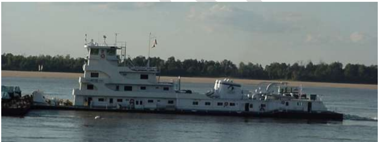
Figure 3-2: Typical 10,500 Horsepower Line Boat
