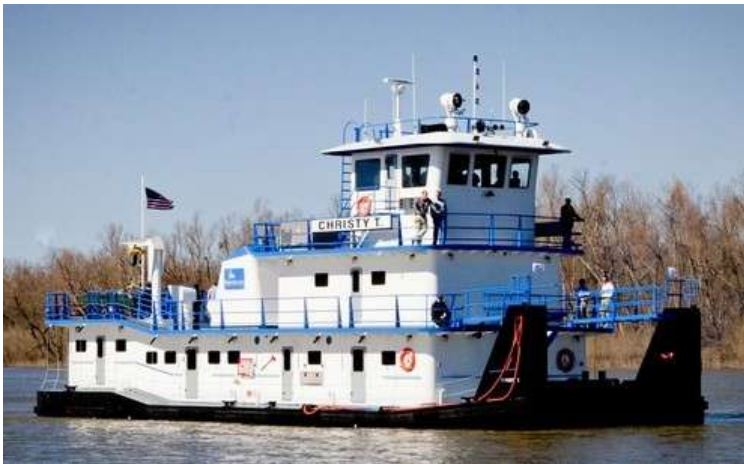
Figure 3-3: Typical 2,000 Horsepower Switch Boat
